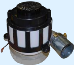
DB9000 Top Motor Ametek #122101-07, 240V, with exhaust tube and carbon capture filter 9065-02 Shipping Wt.: 7 lbs.
